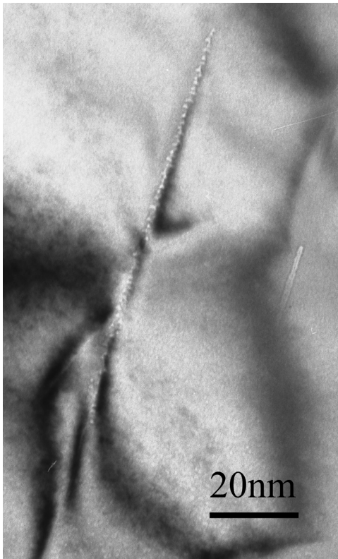
Figure 6 A screw dislocation in HVPE-grown GaN in a cross-sectional sample showing decoration by voids.
